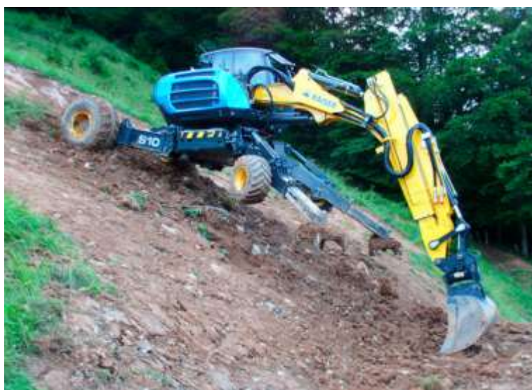
Picture 13. Mechanical excavator adapted for slope works in plantations.
